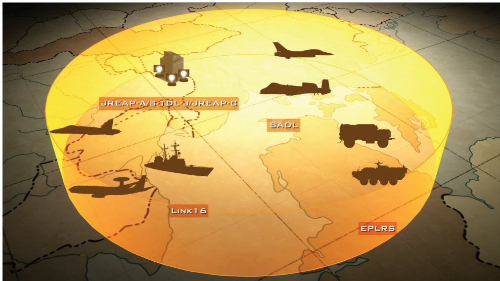
Figure 9-2. When an airborne tactical gateway becomes a participant in the network, that aircraft can be positioned high enough in the sky to maintain line of sight to all participants. This allows the airborne gateway to relay, translate or forward TDL data to all participants, dramatically improving interoperability and communication.
