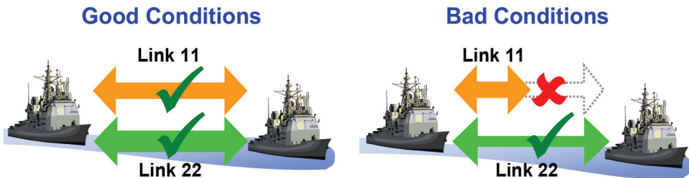
Figure 4-6. Comparison of Link 11 and Link 22 Tactical Data Throughput.
